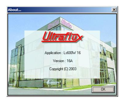
NOTE: Software version of converter (Serial N# <u>xx</u>-yy-zz) must correspond with software version (Version N# Ls600W <u>xx</u>). This underlined 2 numbers must be identical.
