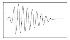
This example shows a thick pipe on which we can use lower frequency probes and also accept some corrosion.
