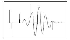
This example shows the benefit of high frequency probes on a thin and clean pipe wall.
