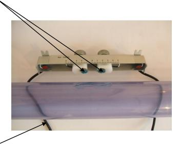
Attach probes to the pipe with straps or better use the probe support.
