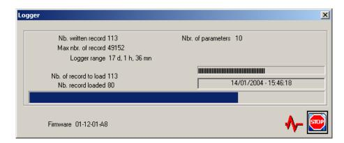
Clicking on Stop closes the file at reached Number / Time. This file is stored "by default" in the data folder with an extension [\*.log]. It is Excel compatible by respecting a [\*.prn] format\_(ASCII + Tab separators).
