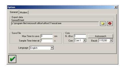
You can adapt the Com. Port Parameters manually as set on UF 801-P, but the easier method is to\_click on **Auto Search**. This searches for the communication settings and the Com Port set by the PC for the USB converter: do a try with UF 801-P at 115 000 and then at 9600 bauds if no result.
