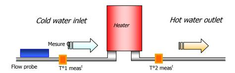
Equipped with this function and two T probes, the UF 801-P measures and displays the two temperatures (inlet and outlet), their difference and compute the energy flow from the raw flow rate and the characteristics of the fluid.
