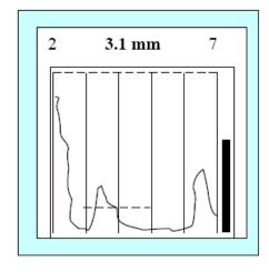
**With the graph**, you can have <u>complementary information</u> on the echo and other conditions attached to the wall thickness: corrosion, including crystallization (as with grey cast iron):
