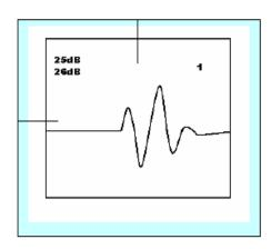
The second screen is an expanded view inside above window that results from the digital acquisition in a tracking window, our electronic lens for ultrasonics.
