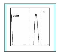
The first one shows, from the left to the right side, all energised signals (ultrasonic, but also noises) that UF 801-P is receiving and must filter and treat.
