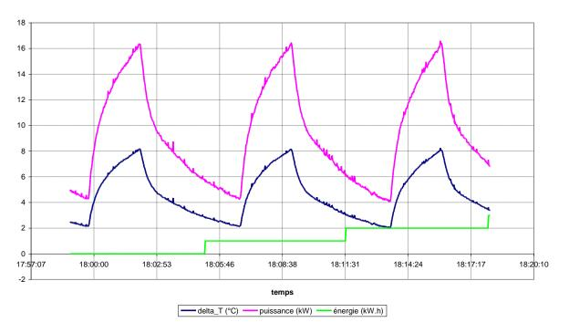
The theoretical power of the heater is 35 kW, but here the peak power is less than 20 kW, with an average power of 8 to 10 kW because gas burning is done during only 30% of the time.
