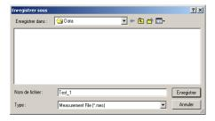
Once the routine is launched, the data are recorded as per the instructions in option menu (sampling rate and recording period). Setting Max. time period = 0 means manual stop (the icon Stop replaces the icon Save).
