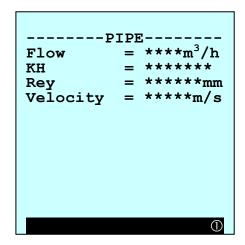
**The flow velocity** informs you about actual conditions compared to the <u>typical</u> <u>flow range of a flow meter</u> (0.5 to 5 m/s).
